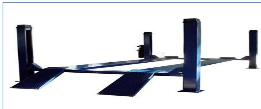
Figure 5.1 Vehicle hoist
